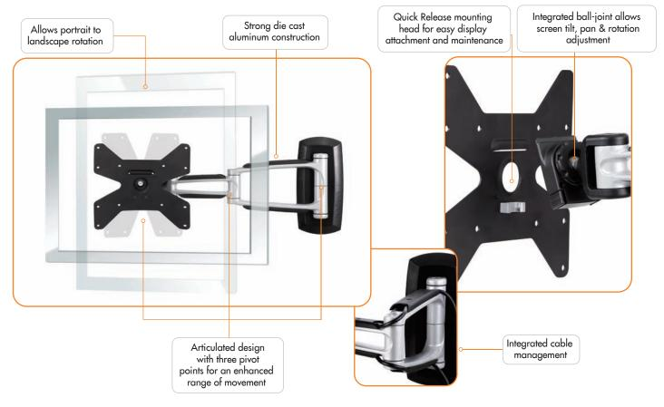
Supports 75x75, 100x100, 200x100 & 200mmx200mm VESA hole patterns. Also supports 200x300, 200x400, 300x200, 300x300, 300x400, 400x200, 400x300 & 400mmx400mm via optional adaptor accessory
