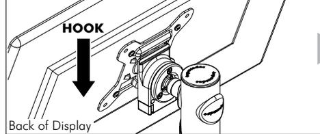
Press and hold the Release Buttons. Gently push bottom of VESA Plate into Quickshift Mount. Release Buttons to lock in place.
