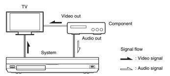
If the component plays sound only, connect the audio output of the component to the system.
