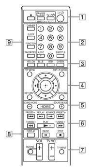
Number 5, AUDIO, VOL +, and ► buttons have a tactile dot. Use the tactile dot as a reference when operating the remote.
