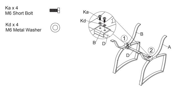
• Hand tighten hardware in sequential order 1 then 2. Don't securely tighten hardware completely.
