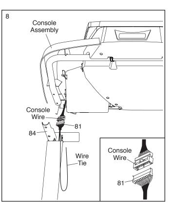
Set the console assembly on the Handrails (84).
