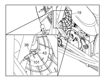
Loosen, but do not remove, the indicated M4 x 16mm Screw (101). Slide the Reed Switch (38) slightly closer to or away from the Magnet (43), and then retighten the Screw. Then, plug in the power cord, press the power switch to the reset position, and rock the Pulley (19) forward and backward just enough that the Magnet passes the Reed Switch repeatedly.
