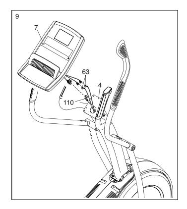
Tip: Avoid pinching the wires. Attach the Console (7) to the Upright (4) with four M4 x 16mm Screws (101); start all the Screws, and then tighten them.
