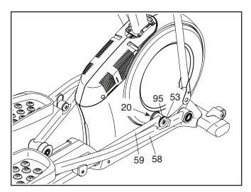
See EXPLODED DRAWING C on page 39. Identify the Left and Right Shields (73, 74). Remove the M4 x 19mm Screws (5) and the M4 x 48mm Screw (107) from the Left and Right Shields. Then, remove the Right Shield.
