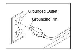
The outlet must be on a nominal 120-volt circuit.
