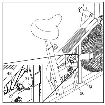
Loosen, but do not remove, the two M4 x 13mm Flange Screws (27). Then, slide the Reed Switch (31) slightly closer to or away from the Magnet (48), and retighten the Screws. Turn the Right Crank Arm (26) for a moment.
