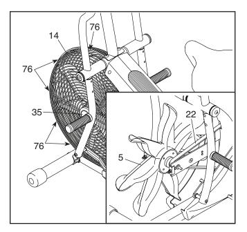
If the Drive Belt (22) needs to be adjusted, first loosen the right Guard Fastener (not shown). To tighten the Drive Belt, turn the M6 Nuts (53) clockwise; to loosen the Drive Belt, turn the M6 Nuts counterclockwise.
