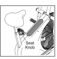
ward slightly to make sure that the pin on the seat knob is engaged in one of the adjustment holes in the seat post. Then, tighten the seat knob.
