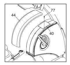
Next, remove the M4 x 16mm Screw (77) from the Access Cover (40) and remove the Access Cover.
