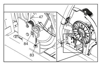
When the drive belt is correctly adjusted, reattach the left and right shields, the top shield, the front shield, the left pedal disc, and the left pedal. Then, plug in the power adapter.
