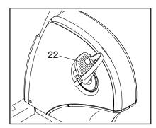
See EXPLODED DRAWING A on page 34. Using a standard screwdriver, gently release the tabs on the Front Shield (58) and the Top Shield (44) and remove them.
