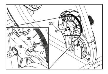
Plug in the power adapter, and turn the Right Crank Arm (23) for a moment. Repeat these actions until the console displays correct feedback.
