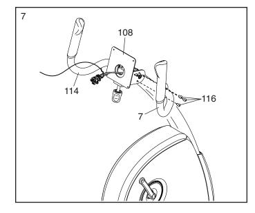
8. Have a second person hold the Console (4) near the Console Bracket (108).
