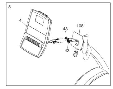
9. **Tip: Avoid pinching the wires.** Attach the Console (4) to the Console Bracket (108) with four M4 x 16mm Screws (77); **start all the Screws, and then tighten them.**
