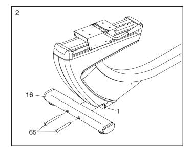
Set a sturdy piece of packing material (not shown) under the front of the Frame (1). Have a second person hold the Frame to prevent it from tipping while you complete this step.
