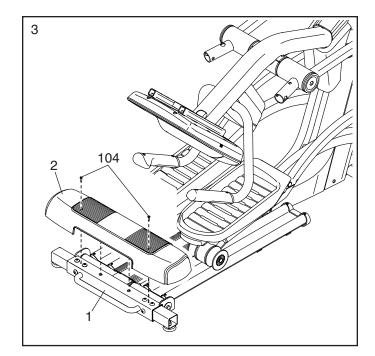
4. With the help of a second person, place some of the packing materials (not shown) under the front of the Frame (1). Have the second person hold the Frame to prevent it from tipping while you complete this step.
