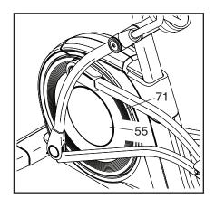
Next, turn the left Crank Arm (20) until one of the Magnets (43) on the Pulley (19) is aligned with the Reed Switch (38). Then, loosen, but do not remove, the two M4 x 16mm Screws (104), slide the Reed Switch slightly closer to or away from the Magnet, and retighten the Screws.
