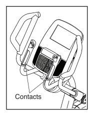
When your pulse is detected, your heart rate will be shown. For the most accurate heart rate reading, hold the contacts for at least 15 seconds.
