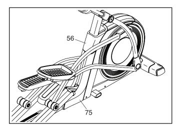
Then, remove the four M4 x 16mm Screws (not shown) from the upper and lower ends of the Rear Shield (75), and remove the Rear Shield.
