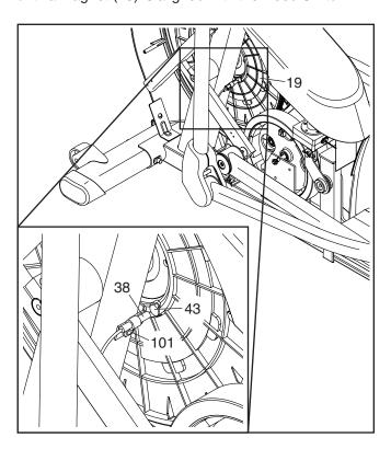
Loosen, but do not remove, the indicated M4 x 16mm Screw (101). Slide the Reed Switch (38) slightly closer to or away from the Magnet (43), and then retighten the Screw. Then, plug in the power cord, press the power switch to the reset position, and rock the Pulley (19) forward and backward just enough that the Magnet passes the Reed Switch repeatedly.
