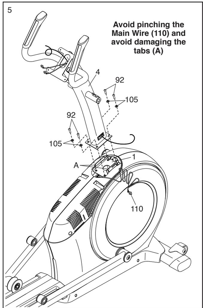
6. Locate the wire tie (B) in the lower end of the Upright (4). Tie the wire tie to the Main Wire (110). Then, pull the upper end of the wire tie until the Main Wire is routed through the Upright.
