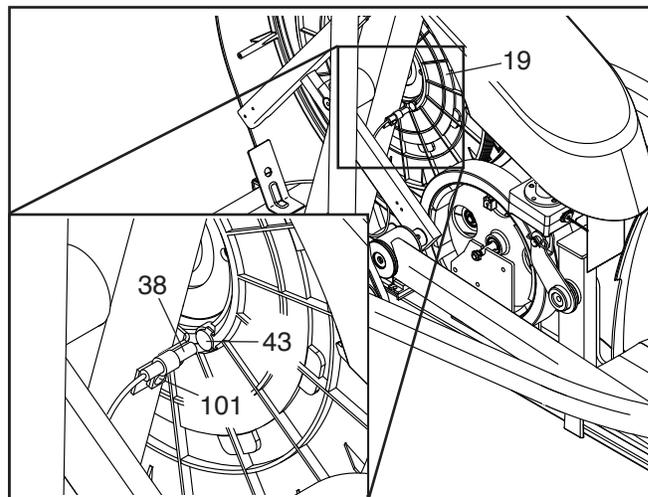
Slightly loosen the indicated M4 x 16mm Screw (101). Slide the Reed Switch (38) slightly closer to or away from the Magnet (43), and then retighten the Screw. Then, plug in the power cord, press the power switch to the reset position, and rock the Pulley (19) forward and backward just enough that the Magnet passes the Reed Switch repeatedly.
