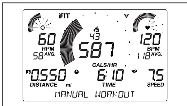
**Calories (flame icon)**—This display will show the approximate number of calories you have burned. When some onboard workouts are selected, this display will show the number of calories remaining to be burned for the workout.
