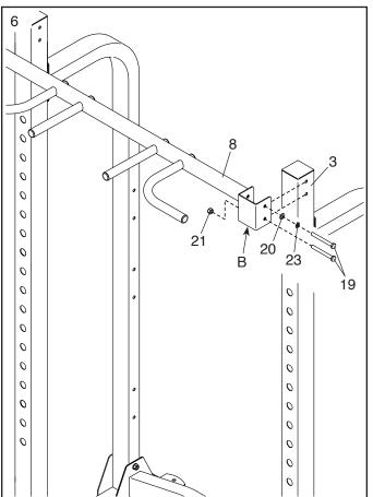
7. See steps 2–6. Tighten all the M10 Locknuts (21), M10 x 95mm Bolts (19), and M10 x 20mm Screws (22).
