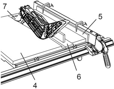
8. Continue pushing the workpiece (4) with the push stick (3) or push block (6 - Fig. RR) until it passes through the blade guard and clears the rear of the table. (Fig. QQ)
