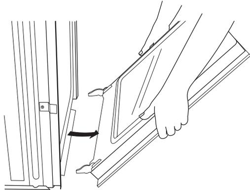
6. Set the oven door(s) aside on the prepared covered work surface, with the oven door resting on its handle.
