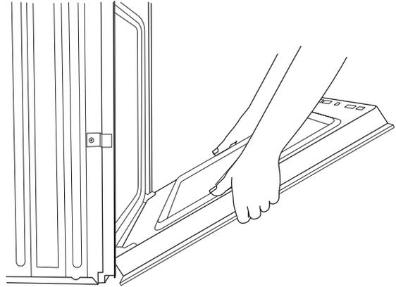
5. Using two hands, grasp the edges of the oven door. Lift and pull the oven door toward you to remove. You may need to gently shift door from side to side as you pull.
