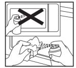
For exterior surfaces and control panel: Use a soft cloth with spray glass cleaner. Apply the spray glass cleaner to the soft cloth; do not spray directly on the oven.
