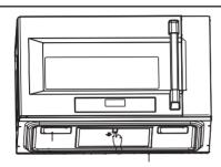
Soak grease filter in hot water and a mild detergent. Scrub and swish to remove embedded dirt and grease. Rinse well and shake to dry. Do not clean filter with ammonia, corrosive cleaning agents, such as lye-based oven cleaners, or place them in a dishwasher. The filters will turn black or become damaged.
