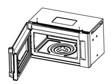
3. Lift the bottom of the charcoal filter. Slide the filter straight out.
