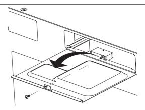
Remove burnt out LED light and replace only with an equivalent 1.5 watt LED light available from parts distributor, the part number is 5304499540.
