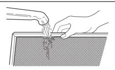
4. To replace grease filter, slide filter in the frame slot on back side of the opening. Push filter upward and lock into place.
