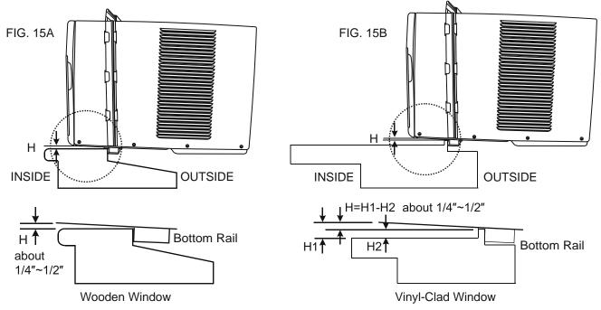
In order to minimize air leaks between the room air conditioner and the window opening, suitable weather stripping(trim the provided weather stripping into suitable size) should be applied in case of any gaps found at the location as indicated by the arrows in Fig. 16.
