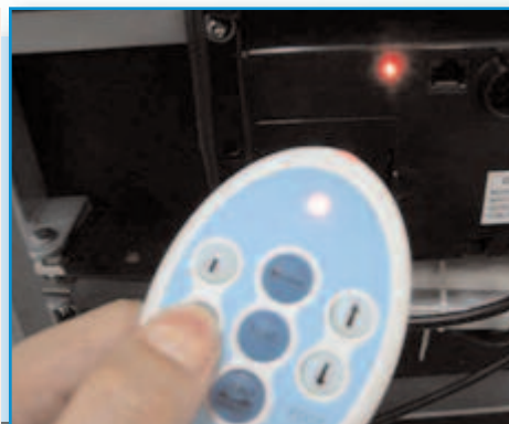
Figure 8: Lower the bed using the 9 volt battery backup system
