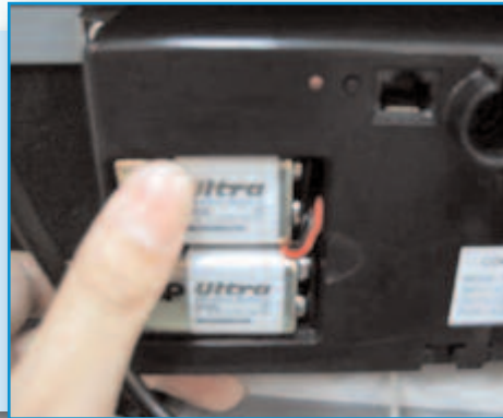
Figure 6: Install the 9 volt batteries
