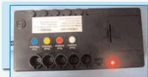
Figure 2: The red LED will light up when the control box is in the learning mode.
