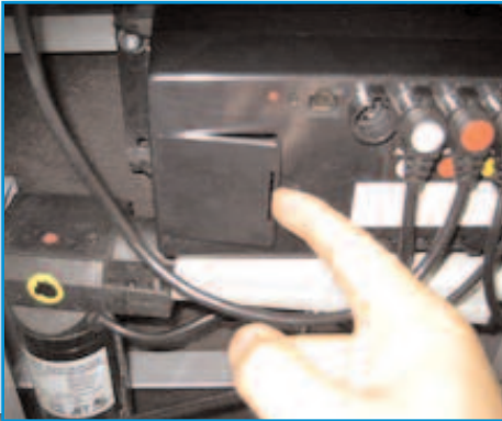
Figure 5: 9 volt battery cover
