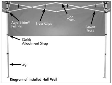
**Step 2.** Attach half wall to frame as shown. (2) Attach quick attachment truss clips around the top truss as shown.
