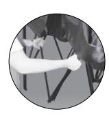
6. With partner on 8' sides, opposite side of shelter, stand facing one another. Grasp the bottom of the diamond shaped area of trusses on opposite sides. Lift up and step backward until shelter is 3/4 opened, being careful not to pinch fingers.
