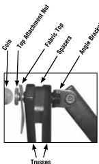
\*5. Unscrew top attachment nut from bolt. Place grommeted fabric top over the bolt, screw on top attachment nut and tighten until snug. Top should rotate easily - do not overtighten. Repeat this procedure on the remaining grommets.
