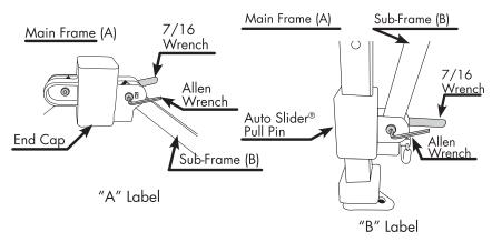
Attach the Main Frame (A) to the Sub-Frame (B) at each of the six connection points:
