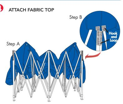
A Gently unfold the fabric top, and place it over the semi-opened frame. Identify the fabric corners and align them with the frame corners.
