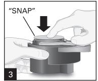
Press down on edge of the pack until the pack snaps into place and hole is punched in the bottom. Do not remove foil.
