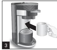
Place a cup underneath to catch the water/vinegar solution.
