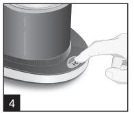
Press the ON/OFF (I/O) button once. After 30 seconds, unplug unit and allow vinegar to clean. After 30 minutes, plug in unit and allow it to finish the brew cycle. When brew cycle is finished, wait for unit to cool. Empty cup and rinse. Repeat steps 1-4 with 1 cup (237 ml) of cold tap water instead of 1/2 cup (118 ml) of vinegar and 1/2 cup (118 ml) of water.
