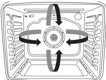
During convection baking or roasting, the bake, broil, and convection elements cycle on and off in intervals while the fan circulates the hot air.
