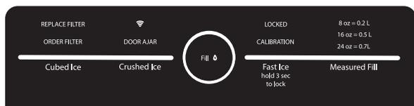
**IMPORTANT:** The display screen on the dispenser control panel will turn off automatically and enter Sleep mode when the control buttons and dispenser paddles have not been used for 2 minutes or more. Touch any control button to reactivate the display screen. The Home screen will appear as shown.
