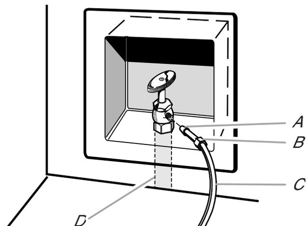
A. Sleeve      C. Copper tubing (to refrigerator)
