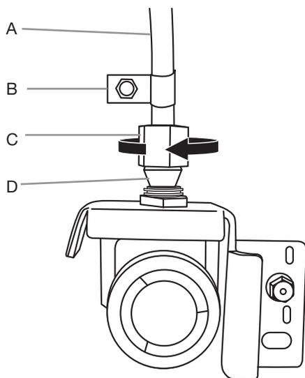
A. Copper tubing    C. Compression nut
