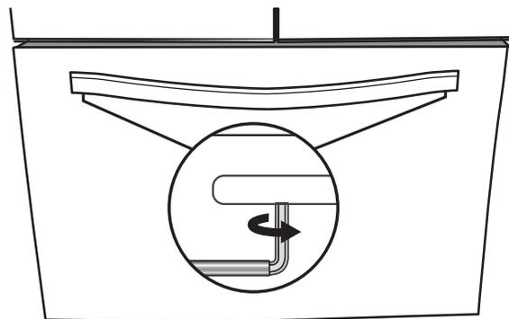
4. Using a left-to-right motion, tighten the setscrew a quarter turn at a time just until it begins to contact the shoulder screw. Do not fully tighten.
