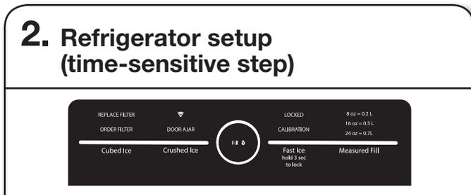
**NOTE:** Step 2 will happen after 30 seconds of power-up. Touch and hold CUBED ICE and CRUSHED ICE together for 3 seconds to enable Wi-Fi.
