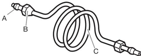
A. Compression sleeve    C. Copper tubing
