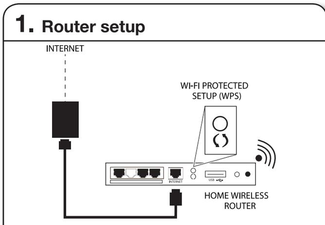
Press the WPS button on the router. An indicator light will begin blinking.
