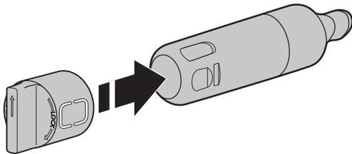
6. Insert the filter into the housing.
