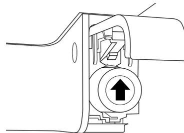
1. Locate the water filter in the top-right corner of the refrigerator compartment.
