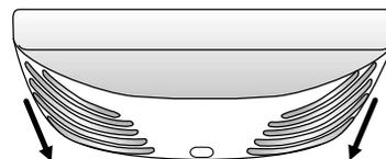
3. Replace the burned-out bulb with an appliance bulb(s) no greater than 25 watts.
