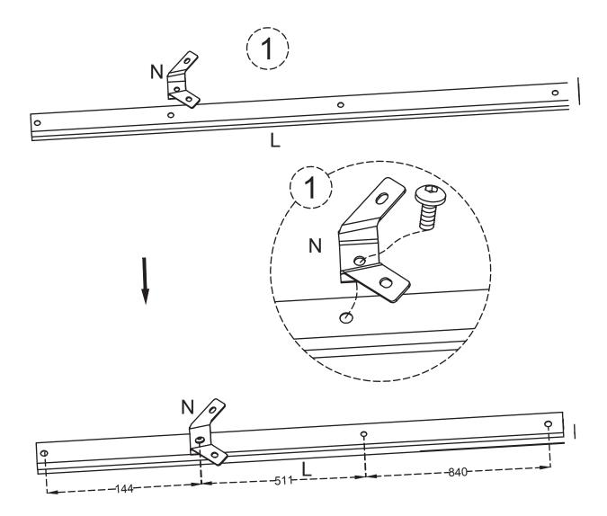
9. Use bolts (AA) secure roof connector (J) with long roof tube (L) as figure 1 shown, then insert bolts (AA) through corner connector (N) of long roof tube (L) secure with post (A) as figure 2 shown.
