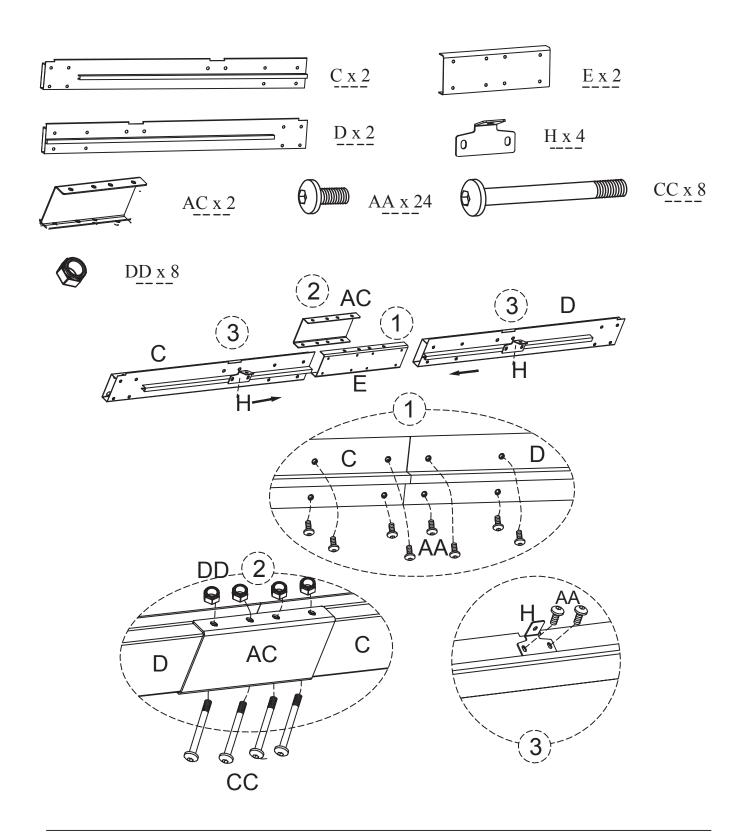
3. Insert inner connector (E) in between short crossbar 1, 2 (F, G) secure with bolts (AA). See figure 1.
