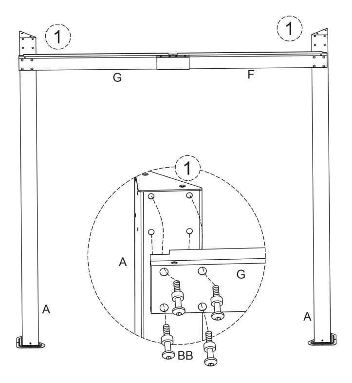
5. Secure the assembled long crossbar set (C, D) with both post (A) by using bolts (BB) as figure 1 shown.
