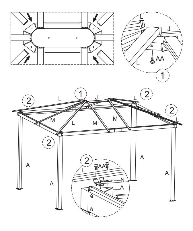
10. Insert bolts (AA) through roof connector (J) underneath secure with roof top cover (K) as figure 1 shown. Don't tighten all bolts before assembly completed.
