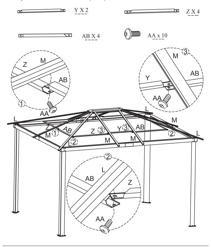
12. Peel off the protection sheet from the panel, then insert roof panel 5 (S) into short roof tube (M) and long roof tube (L), then insert roof panel 6 (T) into short roof tube (M) and long roof tube (L). Repeat the step for remaining roof panels (O, P, Q, R, S, T). Insert bolts (AA) through roof center connector (U) secure with short roof tube (M). Insert bolts (AA) through roof corner connector (V) secure with long roof tube (L). Please do not let the panels slide off.
