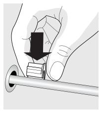
2. Push the shelf grommet onto the wire until it snaps in place.
