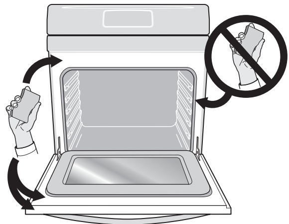
Figure 14: Clean around the oven door gasket
