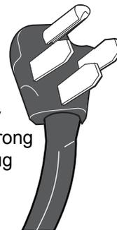
Power supply cord with 4-prong grounding plug
