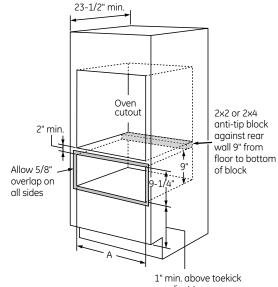
1" min. above toekid or adjust to oven installation height
