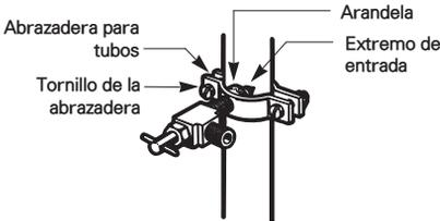
6 ENCAMINE LA TUBERÍA.
