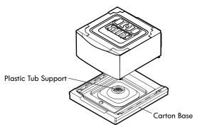
If you must lay the washer down to remove the base packaging materials, always protect the side of the washer and lay it carefully on its side. DO NOT lay the washer on its front or back.
