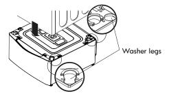
5. Make sure the holes on the pedestal washer align with the holes in the front-loading washer, then install 4 long screws (included in box) at each corner to securely attach the front-loading washer to the pedestal washer.
