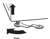
• Turn the locknuts counterclockwise and tighten them when the washing machine is level.
