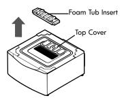
3. Turn the top cover about 180 degrees. Cover the upper hole with the top cover and install 4 short screws (included in packing box) to fix it in place.
