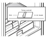
The Glide'N'Serve provides storage space with a variable temperature control that keeps the compartment colder than refrigerator.
