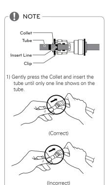
2) Pull the tube to make sure that the tube is tightly fastened and then insert
