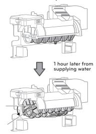
60 minutes after water has been added to the ice tray, the ice tray will sit slightly tilted to help the cold air reach the ice.
