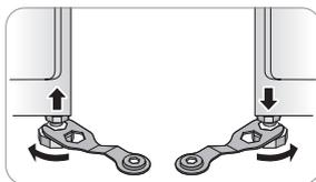
Raise or lower the unit using the leveling feet until the Styler is level from side to side and front to back.
