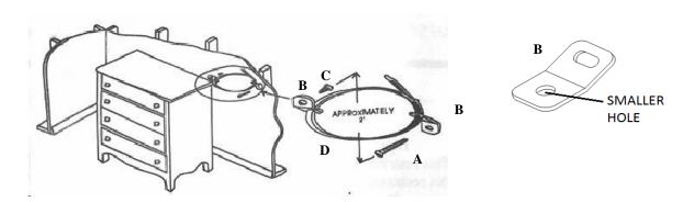
STEP 4: CONFIRM THAT THE STRAP IS SECURELY LACED AND LOCKED.
