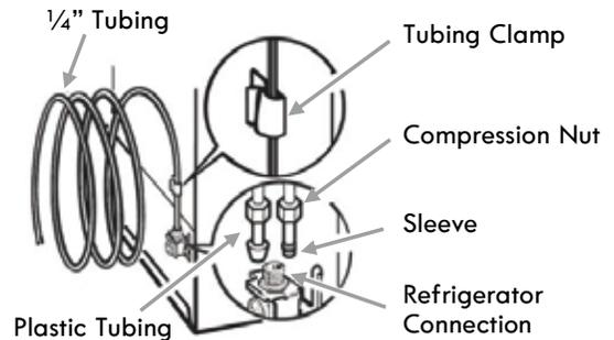
4. Use the tube clamp on the back of the refrigerator to secure the tubing to the refrigerator as shown. This will help avoid damage to the tubing when the refrigerator is pushed back against the wall.
