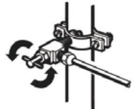
6. Check for leaks. Tighten any connections (including connections at the valve) or nuts that leak.
