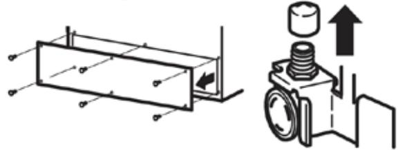
**NOTE:** Be sure to save the screws as the access cover must be reinstalled later to ensure your refrigerator will function properly.
