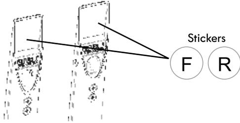
**NOTE:** Before installation, select the proper handle by reading the sticker located here.
