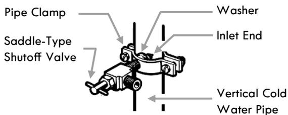
7. Place the compression nut and sleeve for copper tubing onto the end of the tubing and connect it to the shutoff valve. Make sure the tubing is fully inserted into the valve. Tighten the compression nut securely. For plastic tubing, insert the molded end of the tubing into the shutoff valve and tighten compression nut until it is hand-tight; then tighten one additional turn with a wrench. Overtightening may cause leaks.
