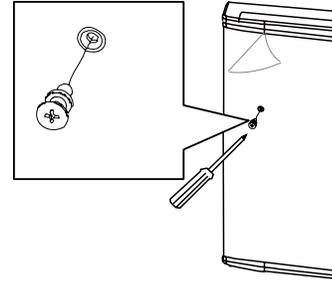
**NOTE:** Remove protective film before installing the handle.
