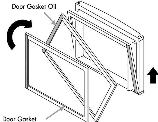
**NOTE:** The oil on the gasket is normal. There is no need to clean the oil. It helps to prevent deformation of the hinge side of gasket. If more oil is needed, use Vaseline.
