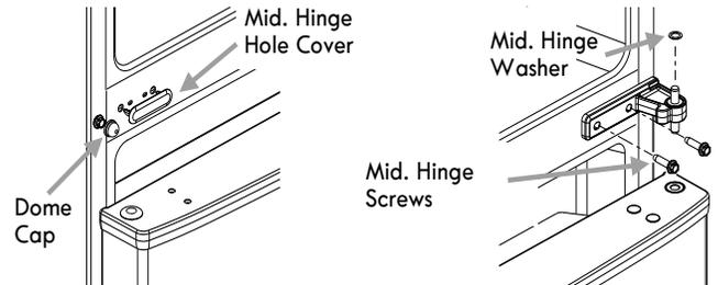
**NOTE:** Do not misplace the middle hinge screws and the middle hinge washer. If the washer is not on the hinge, check to see if it is stuck to the bottom of the door.
