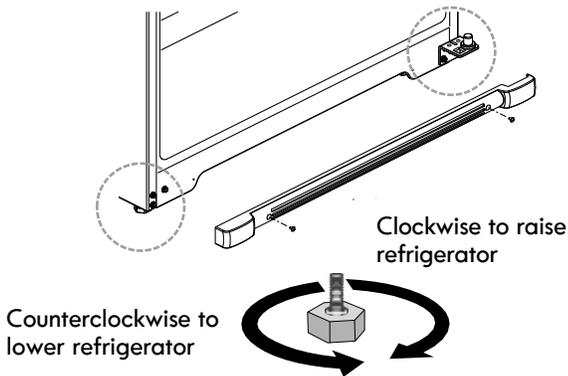
3. Open both doors again to make sure they close as easily as you like and that they stay closed. If not, tilt the refrigerator slightly more to the rear by turning both leveling legs clockwise.
