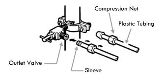
8. Place the free end of the tubing in a container or sink, and turn ON the main water supply. Flush the tubing until water is clear. Turn OFF the shutoff valve on the water pipe. Coil the copper tubing.
