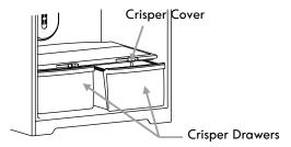
**NOTE:** If the refrigerator door prevents you from taking out a crisper drawer, first try removing any obstructing door bins. If bin removal still does not provide enough clearance, the refrigerator will need to be rolled forward from its installation position until the door can be opened enough to glide the drawers out.
