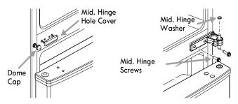
**NOTE:** Do not misplace the middle hinge screws and the middle hinge washer. If the washer is not on the hinge, check to see if it is stuck to the bottom of the door.
