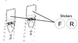
**NOTE:** Before installation, select the proper handle by reading the sticker located here.
