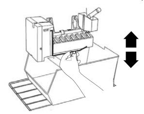
**NOTE:** Turn the icemaker off before removing the ice storage bin to serve ice or to clean the bin. This will keep the ice cubes from dropping out of the icemaker and into the freezer compartment. After replacing the ice storage bin, turn on the icemaker.
