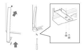
**Step: 3.**Tighten the hex screw in the handles using the hex wrench provided.
