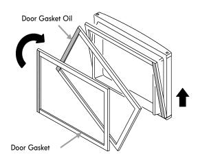
**NOTE:** The oil on the gasket is normal. There is no need to clean the oil. It helps to prevent deformation of the hinge side of gasket. If more oil is needed, use Vaseline.
