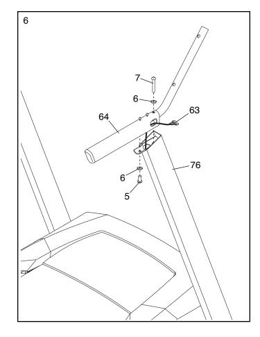
Set the console assembly face down on a soft surface to avoid scratching the console assembly.
