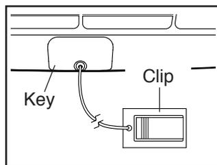
After a moment, the displays will light. **IMPORTANT:** In an emergency, the key can be pulled from the console, causing the walking belt to slow to a stop. Test the clip by carefully taking a few steps backward; if the key is not pulled from the console, adjust the position of the clip.
