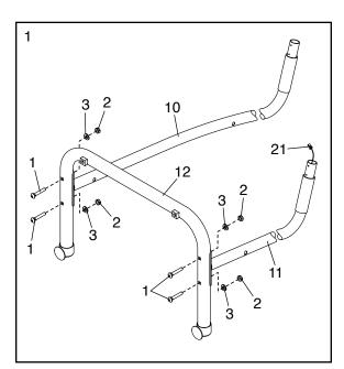
2. Raise the Right Handrail (10) and the Left Handrail (11) to the position shown.
