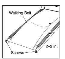
terclockwise 1/4 of a turn. When the walking belt is properly tightened, you should be able to lift each edge of the walking belt 2 to 3 in. (5 to 7 cm) off the walking platform. Be careful to keep the walking belt centered. Walk on the treadmill for a few minutes. Repeat until the walking belt is properly tightened.
