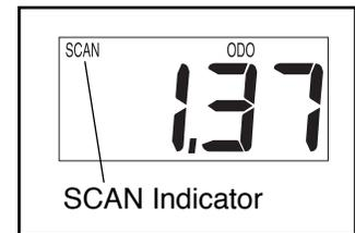
To select only the Speed, Distance, Time, Odometer, or Calorie mode, press the console button until only the SPEED, DIST, TIME, ODO, or CAL indicator appears in the display. Make sure that the SCAN indicator does not appear.
