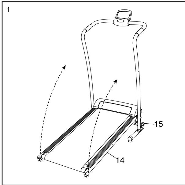
2. Hold the treadmill securely with your left hand as shown. Insert the Pin (15) into the hole in the right side of the Right Handrail (10) and into the Frame (14) as far as it will go.
