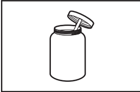
Pipe-joint compound resistant to propane gas
