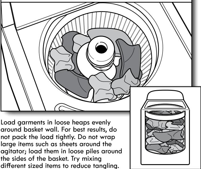
Load garments in loose heaps evenly around basket wall. For best results, do not pack the load tightly. Do not wrap large items such as sheets around the agitator; load them in loose piles around the sides of the basket. Try mixing different sized items to reduce tangling.
