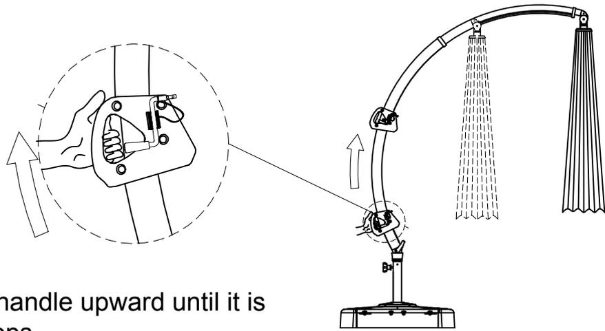
Slide umbrella crank handle upward until it is fully extended and stops.
