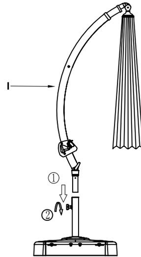
Securely tighten the knob clockwise.
