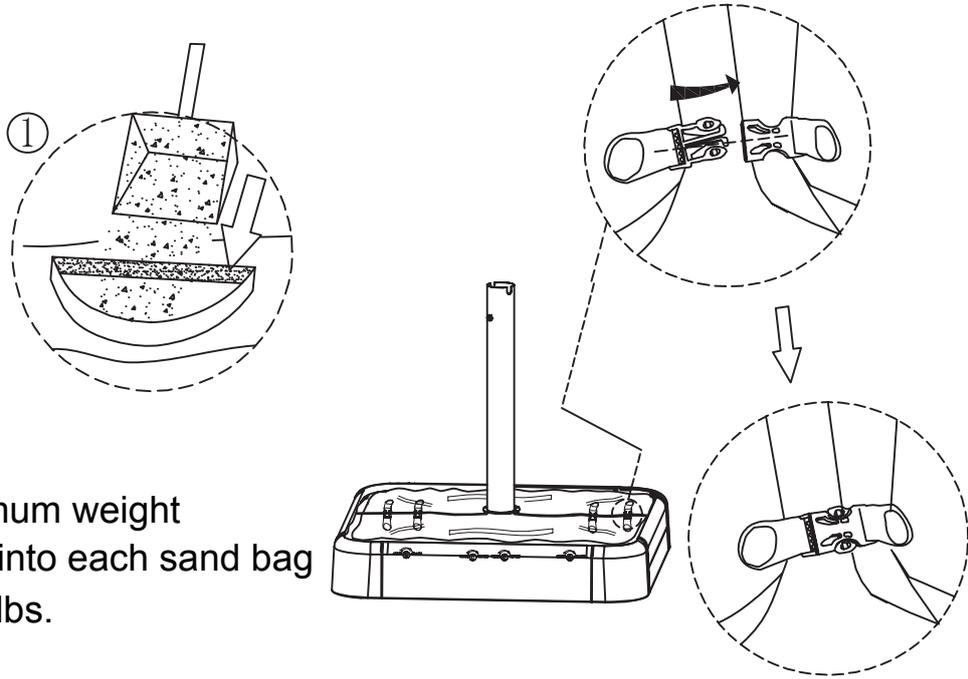
The recommended minimum weight of the sand to be placed into each sand bag is 88lbs for a total of 176lbs.
