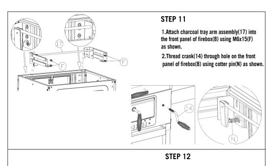
Attach the charcoal tray(16) into the charcoal tray arm assembly(17) using M6 x15 (F) as shown.
