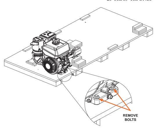
**Step 2.6** Remove Tank & Engine Assembly from crate, then remove the Beam & Cylinder Assembly. Lift Beam & Cylinder Assembly to its vertical position standing on the footplate.
