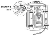
2 Locate the four hole caps included in the accessory pack and install them in the shipping bolt holes.
