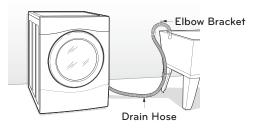
3 Use a tie strap to secure the drain hose in place.
