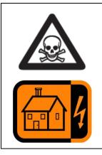
Improper connections to a building electrical system can allow electrical current from the generator to back feed into the utility lines. Such back feed may electrocute utility company workers or others who contact the lines during a power outage, and the generator may explode, burn or cause fires when utility power is restored. Consult the utility company or a qualified electrician.
