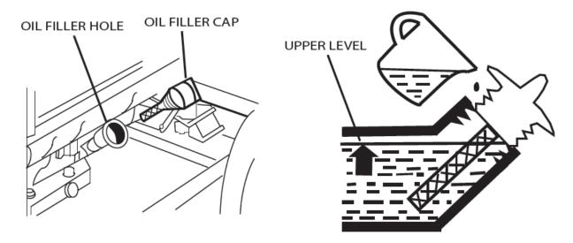
➤ Use only 4-stroke motor oil that meets or exceeds the requirements for API service classification SJ. SAE 10W-30 is recommended for general, all-temperature use. Other viscosities shown in the chart may be used when the average temperature in your area is within the indicated range.
