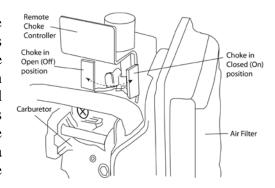
engine has started and is running steadily, the choke should be opened (disengaged) by turning the lever as far as it will easily go clockwise (away from the air filter).
