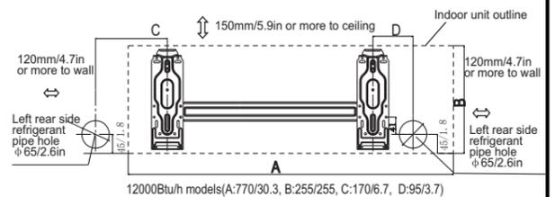
Correct orientation of Installation Plate
