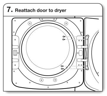
Using a TORX T25  $^{\rm @}$  screwdriver, reinstall the 4 screws securing the door hinge to the dryer.
