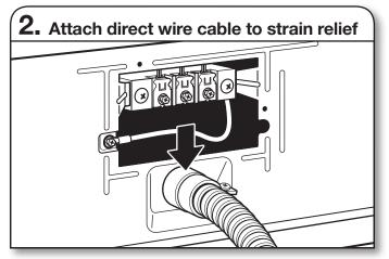
Put direct wire cable through the strain relief. The strain relief should have a tight fit with the dryer cabinet and be in a horizontal position. Tighten strain relief screw against the direct wire cable.
