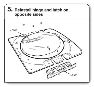
Using a TORX T25 $^{\odot}$  screwdriver, reinstall the latch plate and hinge assembly on the opposite sides from which they were removed.
