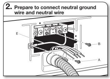
Remove center terminal block screw (B). Remove neutral ground wire (E) from green external ground conductor screw (A).
