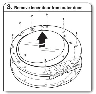
Position the door with the inside of the door facing up. Using a Phillips screwdriver, remove the 10 screws securing the inner door to the outer door. Lift off the inner door and set aside.
