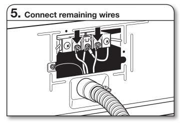
Place hooked ends of remaining direct wire cable wires under outer terminal block screws (hooks facing right). Squeeze hooked ends together and tighten screws. Finally, reinsert tab of terminal block cover into slot of dryer rear panel. Secure cover with hold-down screw. Now, go to "Venting Requirements."
