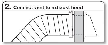
Vent must fit over the exhaust hood. Secure vent to exhaust hood with 4" (102 mm) clamp. Run vent to dryer location using straightest path possible. Avoid 90° turns. Use clamps to seal all joints. Do not use duct tape, screws, or other fastening devices that extend into interior of vent to secure vent, because they can catch lint.
