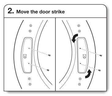
Using a TORX T25<sup>®</sup> screwdriver, remove the 2 screws securing the door strike to the door frame of the dryer. Rotate the strike 180° and attach to the opposite side of dryer door frame, as shown.
