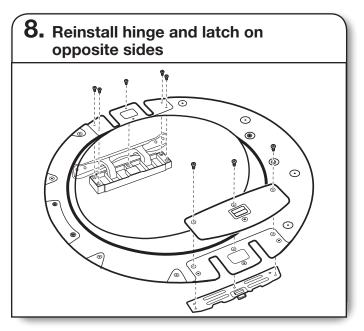
Using a TORX T25<sup>®</sup> screwdriver, reinstall the latch plate, latch backing plate, and hinge assembly on the opposite sides from which they were removed.
