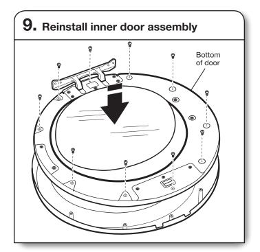
Position the door with the inside of the door facing up. Reinstall the 10 screws securing the inner door to the outer door.
