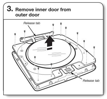
Position the door with the inside of the door facing up. Using a Phillips screwdriver, remove the 13 screws securing the inner door to the outer door. Lift off the inner door and set aside.
