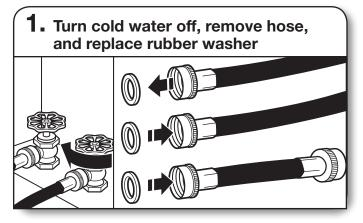
Turn cold water faucet off and remove washer inlet hose. Remove old rubber washer from inlet hose and replace with new rubber washer.
