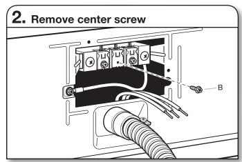
Remove center terminal block screw (B).
