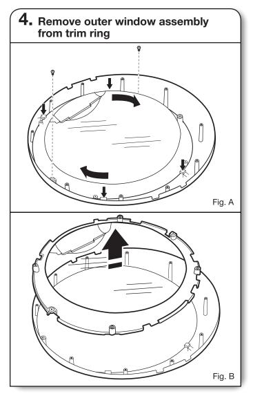
Using a Phillips screwdriver, remove the 2 screws from the outer window retainer and rotate the outer window assembly clockwise until the square notches line up with the 4 tabs on the trim ring indicated with arrows in the figure A above. Then lift out the outer window and retainer up and off the trim ring and set aside (B).
