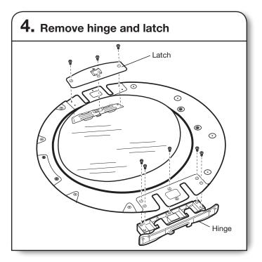
Using a TORX T25<sup>®</sup> screwdriver, remove the 3 TORX<sup>®</sup> screws securing the latch plate and latch backing plate and the 5 screws holding the hinge assembly in place.
