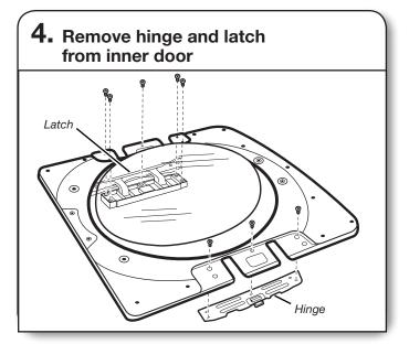
Using a TORX T25<sup>®</sup> screwdriver, remove the 3 TORX<sup>®</sup> screws securing the latch plate and the 5 screws holding the hinge assembly in place.
