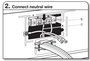
Connect neutral wire (white or center) (C) of power supply cord under center terminal block screw (B). Tighten screw.
