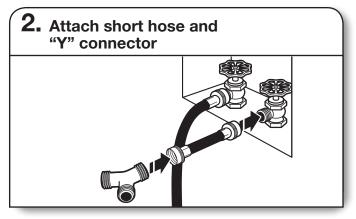
Attach 2 ft (0.6 m) inlet hose to cold water faucet. Screw on coupling by hand until it is seated on faucet. Then attach "Y" connector to male end of the 2 ft (0.6 m) inlet hose. Screw on coupling by hand until it is seated on connector.
