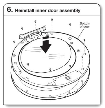
Position the door with the inside of the door facing up. Reinstall the 10 screws securing the inner door to the outer door.
