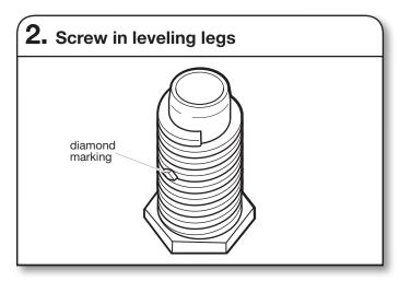
Examine leveling legs, find diamond marking. Screw legs into leg holes by hand – use a wrench to finish turning legs until diamond marking is no longer visible.
