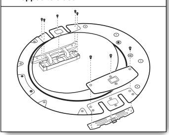
Using a TORX T25<sup>®</sup> screwdriver, reinstall the latch plate and latch backing plate with the 3 TORX<sup>®</sup> screws removed earlier and the hinge assembly with the 5 screws on the opposite sides from which they were removed.
