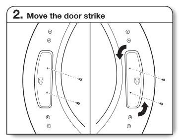
Using a TORX T25<sup>®</sup> screwdriver, remove the 2 screws securing the door strike to the door frame of the dryer. Rotate the strike 180° and attach to the opposite side of dryer door frame, as shown.
