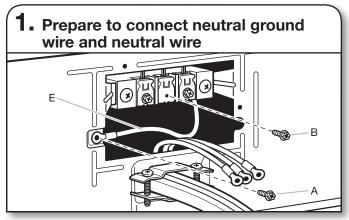
Install the correct strain relief for your electrical connection method, as shown on page 8 or 10.
