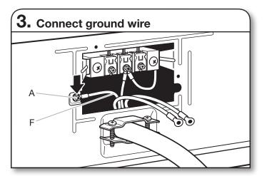
Connect ground wire (F) (green or bare) of power supply cord under green external ground conductor screw (A). Tighten screw.
