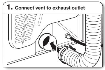
Using a 4" (102 mm) clamp, connect vent to exhaust outlet in dryer. If connecting to existing vent, make sure vent is clean. Dryer vent must fit over dryer exhaust outlet and inside exhaust hood. Check that vent is secured to exhaust hood with a 4" (102 mm) clamp.
