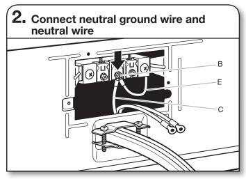
Connect neutral ground wire (E) and neutral wire (white or center wire) (C) of power supply cord or cable under center, terminal block screw (B). Tighten screw.
