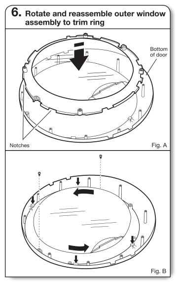
With the edge with 2 notches at the top, align the notches on the outer window assembly with the tabs on the trim ring and lower into place as shown in figure A.
