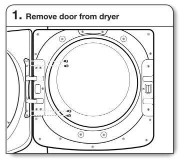
Using a TORX T25<sup>®</sup> screwdriver, remove the 4 screws securing the door hinge to the dryer and lift up and out to remove the door. Place the door on a soft towel or other non-scratch surface. Retain or set aside the 4 screws.
