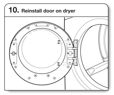
Using a TORX T25<sup>®</sup> screwdriver, remove the 4 screws on the dryer. Insert the tabs on the hinge into the mounting slot and slide down to engage the top tab. Secure in place with the 4 TORX T25<sup>®</sup> screws removed earlier.
