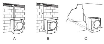
A. Standard rear offset exhaust installation
