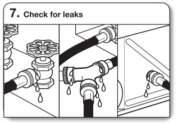
Check for leaks around "Y" connector, faucet, and hoses.
