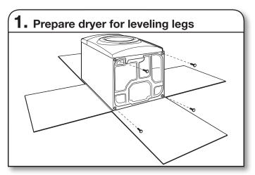
To avoid damaging floor, use a large flat piece of cardboard from dryer carton; place under entire back edge of dryer. Firmly grasp dryer body (not console panel) and gently lay dryer down on cardboard.
