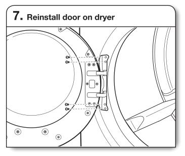
Using a TORX T25<sup>®</sup> screwdriver, remove the 4 screws on the dryer. Insert the tabs on the hinge into the mounting slot and slide down to engage the top tab. Secure in place with the 4 TORX T25<sup>®</sup> screws removed earlier.
