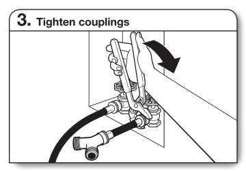
Using pliers, tighten the couplings with additional two-thirds turn.
