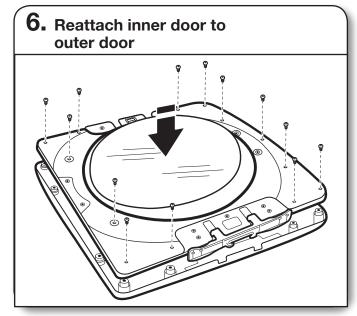
Position the inner door on the outer door assembly. Using a Phillips screwdriver, secure with the 13 screws removed earlier.
