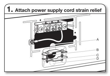
Remove the screws from a 3/4" (19 mm) UL listed strain relief (UL marking on strain relief). Put the tabs of the two clamp sections (C) into the hole below the terminal block opening (B) so that one tab is pointing up (A) and the other is pointing down (D), and hold in place. Tighten strain relief screws just enough to hold the two clamp sections (C) together.
