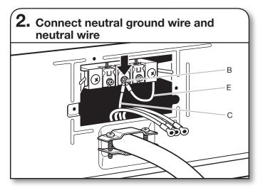
Connect neutral ground wire (E) and neutral wire (white or center) (C) of power supply cord under center terminal block screw (B). Tighten screw.
