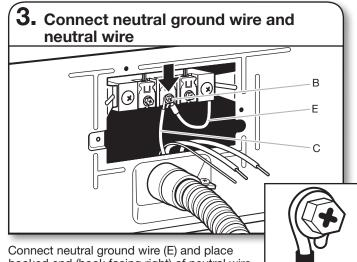
Connect neutral ground wire (E) and place hooked end (hook facing right) of neutral wire (white or center wire) (C) of direct wire cable under center screw of terminal block (B). Squeeze hooked ends together and tighten screw.
