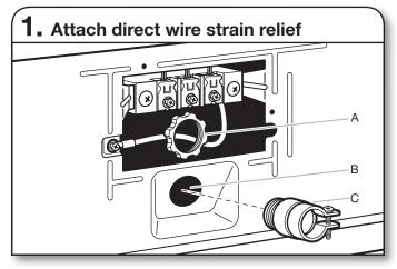
Unscrew the removable conduit connector (A) and any screws from a 3/4" (19 mm) UL listed strain relief (UL marking on strain relief). Put the threaded section of the strain relief (C) through the hole below the terminal block opening (B). Reaching inside the terminal block opening, screw the removable conduit connector (A) onto the strain relief threads and tighten securely.
