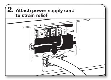
Put power supply cord through the strain relief. Be sure that the wire insulation on the power supply cord is inside the strain relief. The strain relief should have a tight fit with the dryer cabinet and be in a horizontal position. Do not further tighten strain relief screws at this point.
