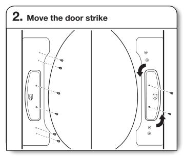
Using a TORX T25<sup>®</sup> screwdriver, remove the 2 screws securing the door strike to the door frame of the dryer. Remove the 4 screws above and below the door strike and set aside for later use. Rotate the strike 180° and attach to the opposite side of dryer door frame, as shown.
