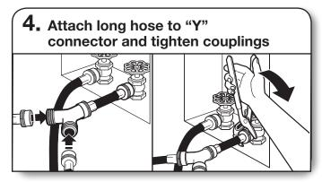
Attach one of the 5 ft (1.5 m) inlet hose ends to the "Y" connector. Attach washer cold inlet hose to other side of "Y" connector. Screw on coupling by hand until it is seated on connector. Using pliers, tighten the couplings an additional two-thirds turn.
