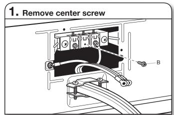
Remove center terminal block screw (B).
