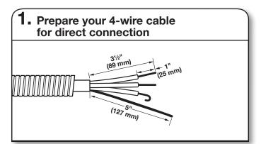
Direct wire cable must have 5 ft. (1.52 m) of extra length so dryer may be moved if needed.
