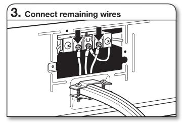
Place ends of remaining wires under outer terminal block screws. Tighten screws.
