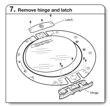
Using a TORX T25<sup>®</sup> screwdriver, remove the 3 TORX<sup>®</sup> screws securing the latch plate and latch backing plate and the 5 screws holding the hinge assembly in place.
