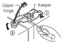
3) Remove the refrigerator compartment door by lifting it up.
