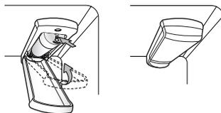
3. After the water filter is replaced, dispense 2.5 gallons of water (flush for approximately 5 minutes) to remove trapped air and contaminants from the system. Do not dispense the entire 2.5 gallon amount continuously. Depress and release the dispenser pad for cycles of 30 seconds ON and 60 seconds OFF.
